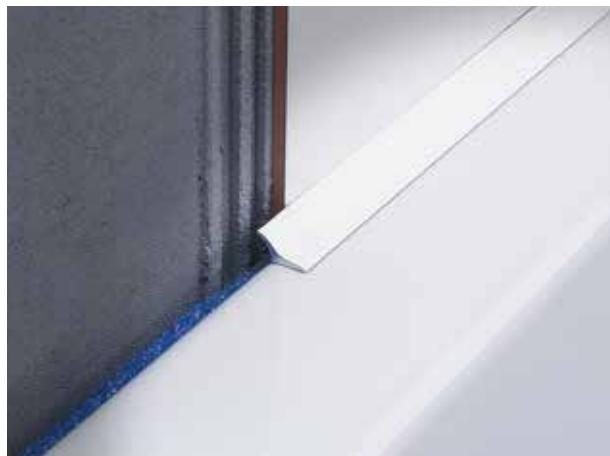
SANITEC SB profiles resolve wall-to-wall or wall-to-floor transitions. The cove-shaped profile is easy to clean and offers a hygienic solution to internal corners in kitchen countertops, shower stalls and bathtubs, replacing silicone caulking that inevitably yellows and absorbs dirt over time. Installed with self-adhesive strips or silicone.
